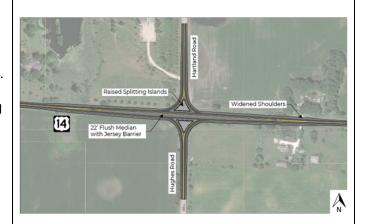
Roundabout: The Roundabout Alternative consists of removing the existing roadway at the intersection of US Route 14 and Hartland/Hughes Road and constructing a roundabout to address safety and speeding concerns. This alternative would consist of widened shoulders, raised islands, a roundabout with an inscribed diameter of 110', truck aprons maintaining passage of trucks, and drainage improvements to account for road widening.
